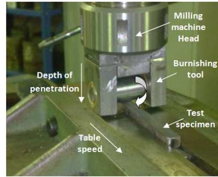
Fig. 4. Mounting of roller burnishing tool on the universal milling machine
