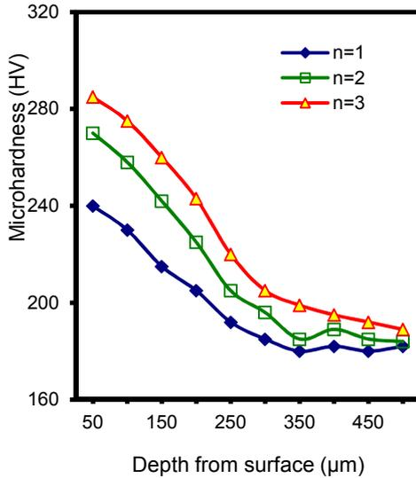
Fig. 8. Microhardness distribution across the subsurface layer
