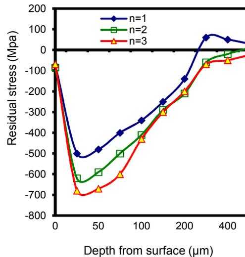
Fig. 10 Residual stress distribution along the subsurface layers for different number of passes
