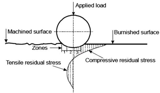
Fig. 2. Schematic representation of the residual stress distribution in the burnishing process [5]
