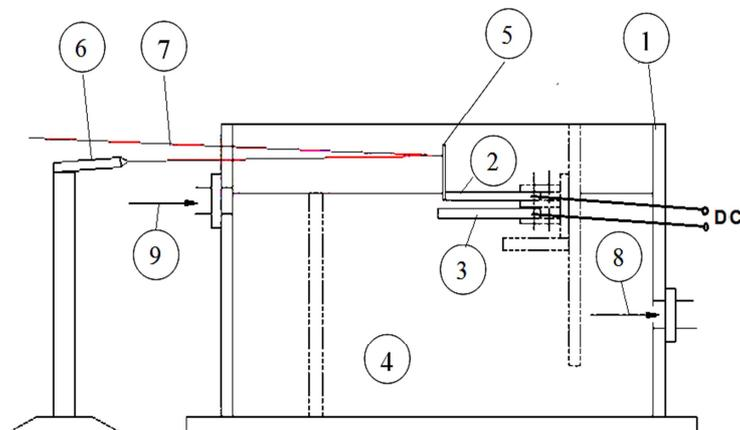
(1)Tank, (2) test specimen, (3) etching tool, (4) electrolyte, (5) mirror, (6) laser pointer, (7) reflecting laser light, (8) electrolyte exit, (9) electrolyte inlet
