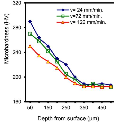
Fig. 9. Effect of burnishing speed on microhardness of subsurface layer
