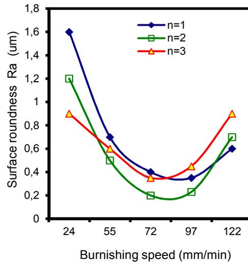
Fig. 7. Effect of burnishing speed on surface roughness at different number of passes
