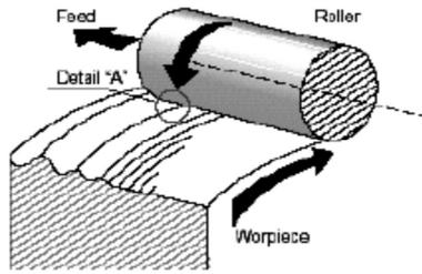
Fig. 1. Roller burnishing process [3]
