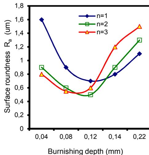
Fig. 6. Effect of burnishing depth on surface Roughness at different number of passes
